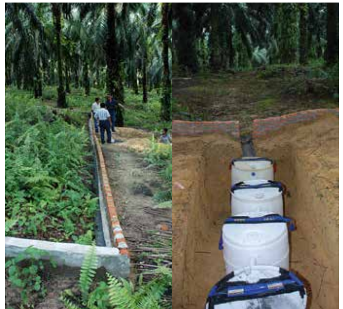
Field design to study soil run-off and erosion in plots with vegetation cover and bare ground.
