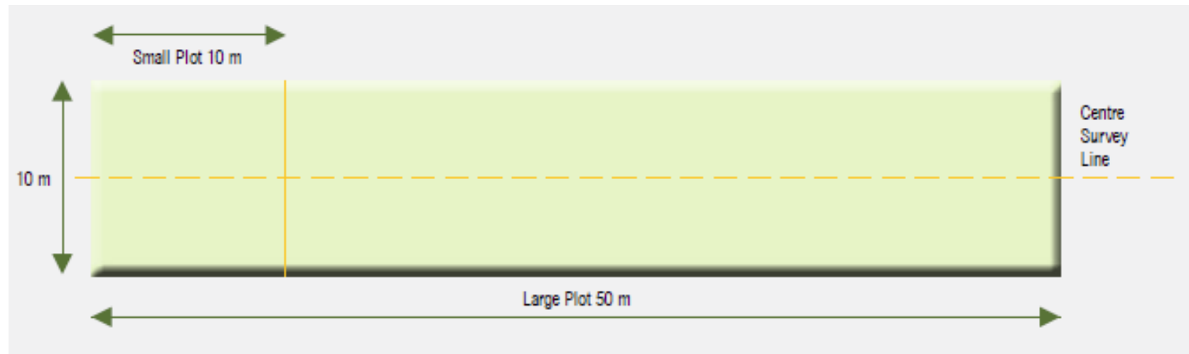
Schematic of the plot design used during the field inventory
